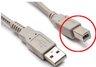
Fig. 50—Plug the USB-B (red) connector into the port on the back of the EVOM3.
