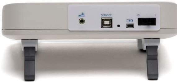
Fig. 4—Foot switch, Future expansion, reset, power connection, power switch
