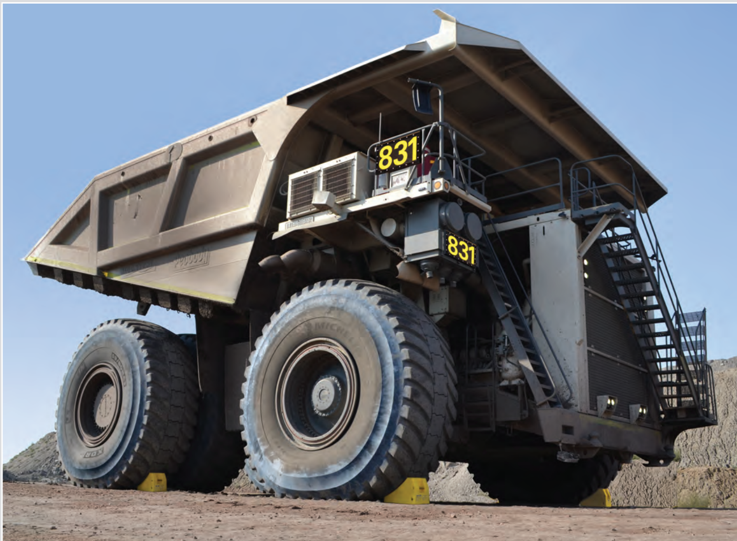
Four Monster wheel chocks, model MC3011 used on Liebherr 400-ton Haul Truck
