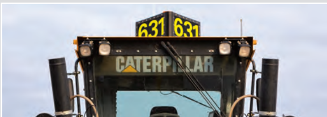
AID™ Triangular Vehicle Identification Light on a road maintenance vehicle.
