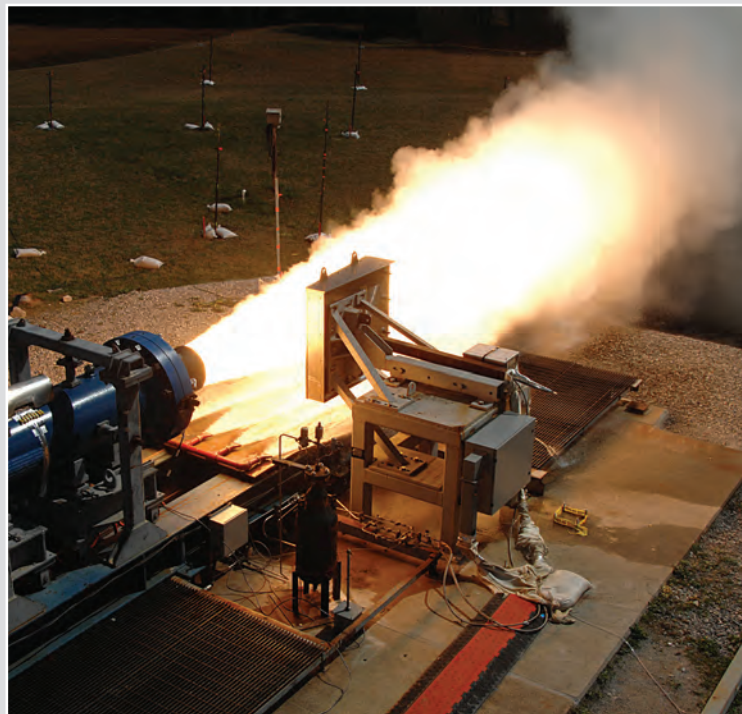
Guard Dog in use during a NASA brilliant sub-scale solid rocket motor test (Photo by NASA)
