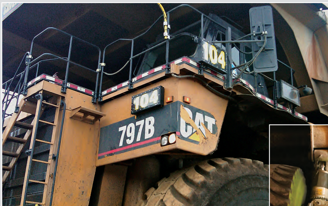
AID™ Rectangular Vehicle Identification Lights on the front of a 400-ton mine haul truck.
