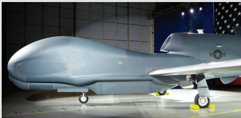
Monster Aviation Chock model AC6820-LR-RP being used with the Global Hawk UAV
