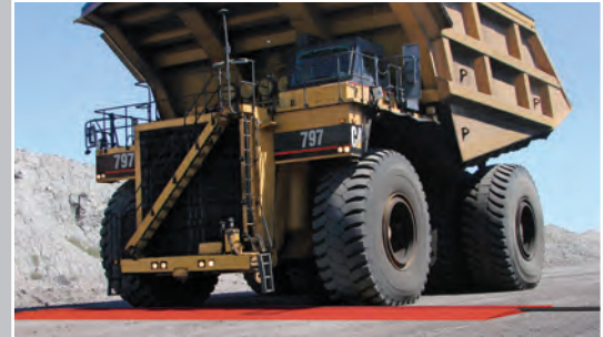
400-ton haul truck drives over an Extreme Crossover Pad
