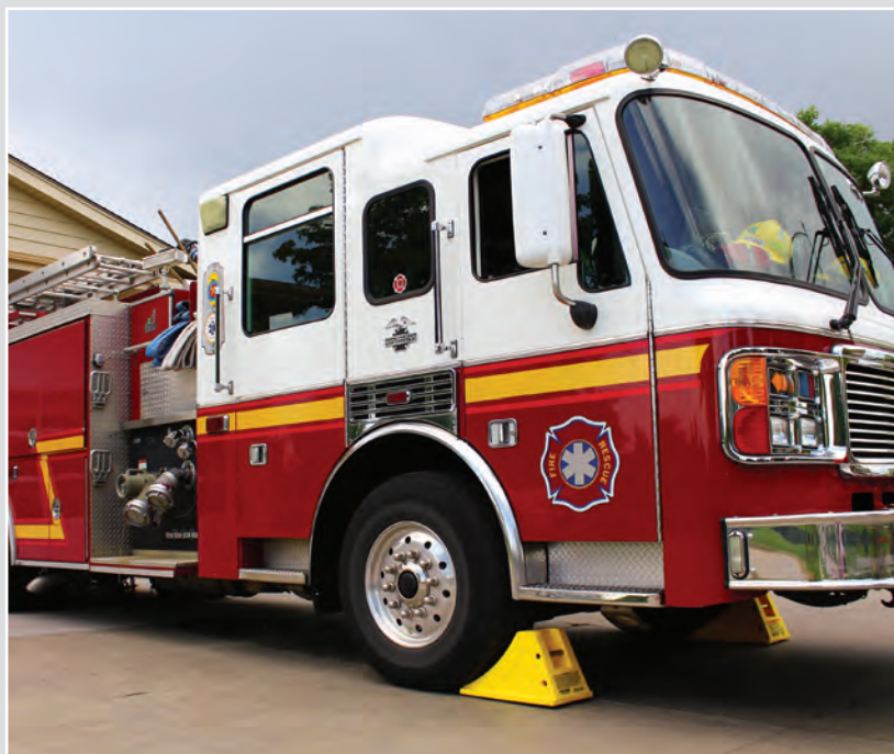
Monster all-terrain chocks model AT3514 used on a fire fighting truck
