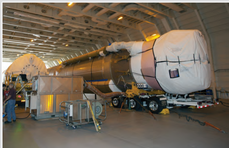
Monster MC Chocks used at NASA to hold the Atlas V launch vehicle. (Photo by NASA)
