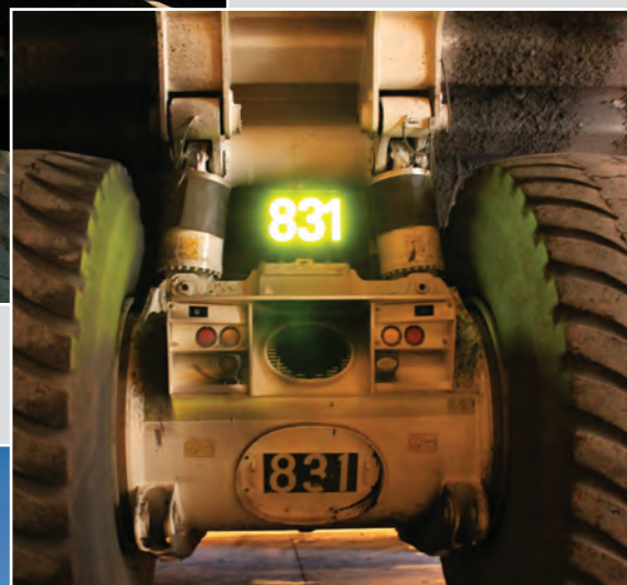
AID™ Rectangular Vehicle Identification Light on the back of a 400-ton mine haul truck.
