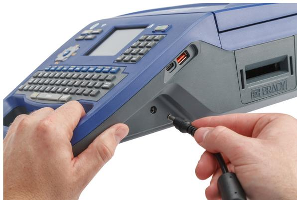
3. Plug the other end of the cord into an electrical outlet.
