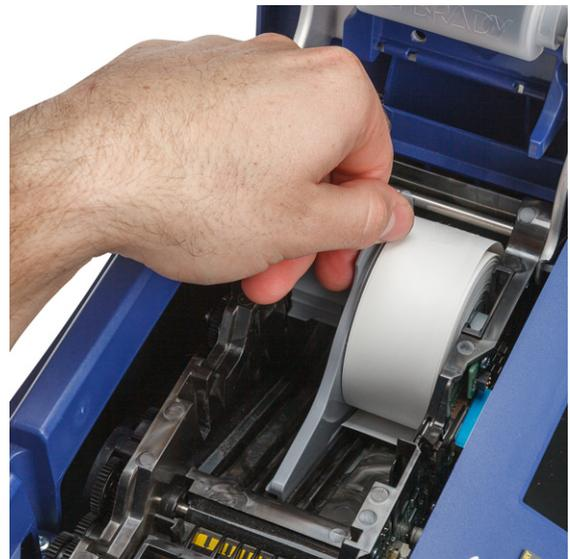
4. Insert the loose label end up to the black line under the ribs, making sure that the label material covers the sensors and that the edge of the label supply roughly aligns with the side of the label well.
