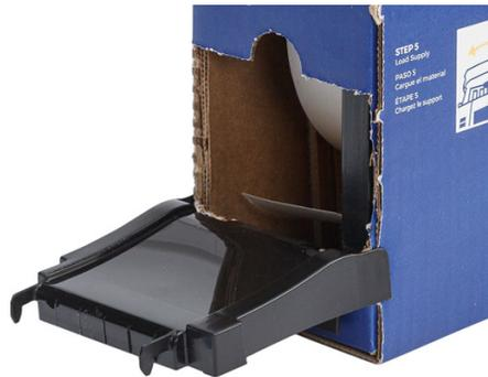
4. Attach the ramp hooks to the outside of the bulk label feed path on the printer.
