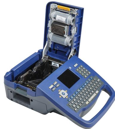
2. Remove the existing ribbon cartridge, if installed. Grasp the finger tabs on either side of the cartridge and pull the cartridge out of the ribbon compartment.
