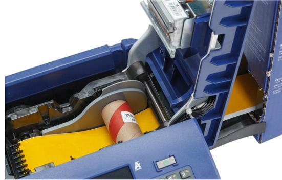
7. Continue to feed the leading edge of the label roll under the core. Insert the loose label end up to the black line under the ribs, making sure that the label material covers the sensors and that the edge of the label supply roughly aligns with the side of the label well. See [Figure 2-1](#) and [Figure 2-2](#) on page 18.
