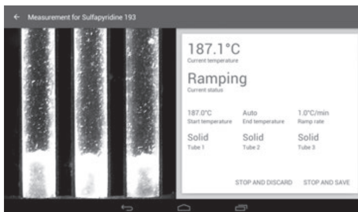
Run screen status 'Ramping'
