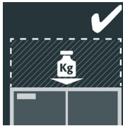
6 Load permitted: An additional cabinet may be placed on the cabinet ceiling.
