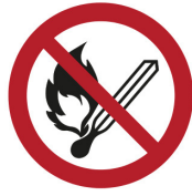
1 Prohibition sign: No open flame
