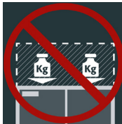
5 Load is prohibited: No additional cabinet may be placed on the cabinet ceiling.
